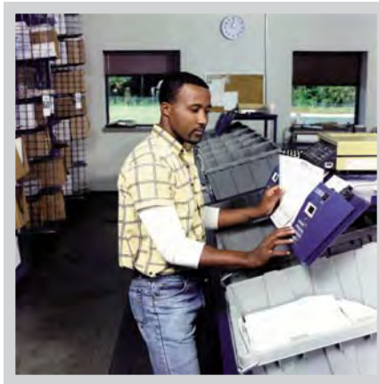
Each item’s location is printed on the order by the host computer and is then keyboarded into the carousel system. The carousels then bring the items to the picker. No walk or search.
