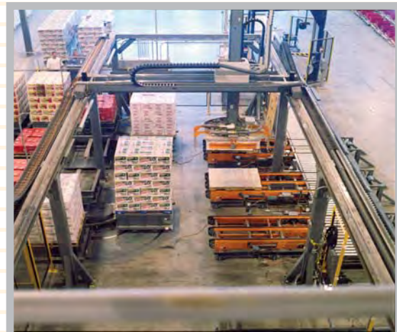
Two Whites' pallet carousels are used with Alvey's gantry robot
