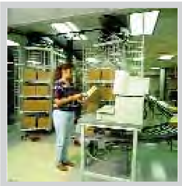
Put system operator scans the carton upon arrival from the first vault.
