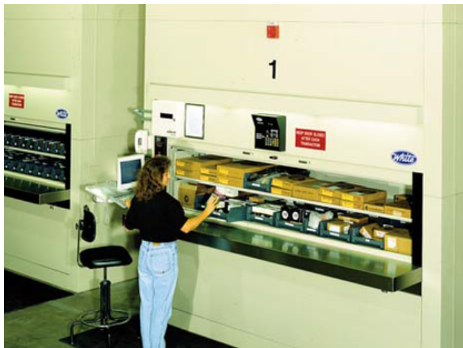
Desired items are presented for picking at an ergonomic level.
