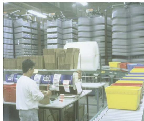
When batch picks are completed, totes move to a waiting conveyor which delivers them to the packing station.
