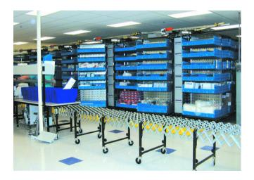
To improve space utilization and picking efficiency for their medical supplies, the company installed 2 pods of 4 horizontal carousel systems equipped with Spectrum Plus software from White Systems.
