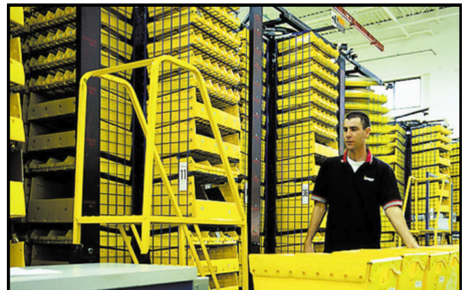
Orders are picked into assigned totes as directed by a lighted Sortbar.
