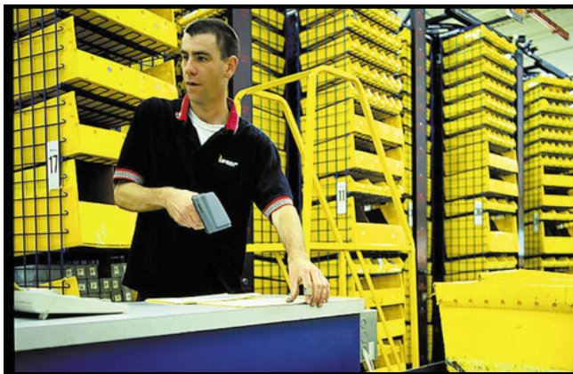
Orders are downloaded to the PC and sorted by ship method. A pick ticket is printed and scanned to set up batches of 16.
