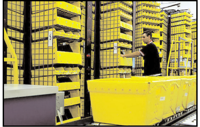
Software optimizes the batches to minimize carousel rotation and lights the Lighttree to indicate position and quantity of item to be picked.
