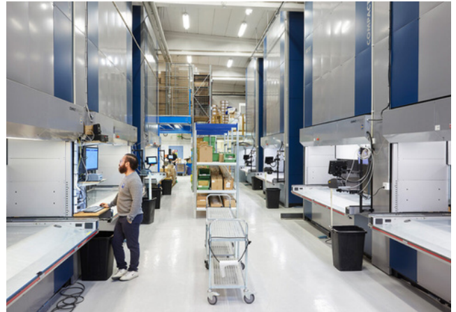
Everything from small screws to exclusive autopilots as big as moving boxes are stored in the VLMs
